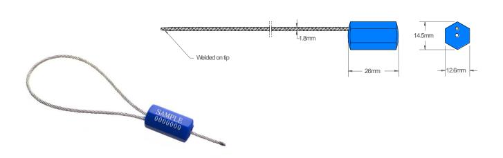
The Acme **CS3 Cable Seal** is a variable length cable seal manufactured from high quality materials. The locking mechanism is protected with a high-impact ABS plastic and the cable is manufactured from galvanized steel. The cable has a welded tip for ease of locking and should the cable be cut it unravels making it impossible to re-lock the seal again without showing obvious signs of tampering. The seal requires cutters for removal.
