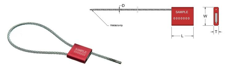
The Acme **CS1 Cable Seal** is available in various cable lengths and diameters to suit all requirements. The lock body is manufactured from die-cast aluminum and the cable from non-preformed galvanized steel. The cable has a welded tip for ease of locking and should the cable be cut it unravels making it impossible to re-lock the seal again without showing obvious signs of tampering. The cable seal require cutters for removal.
