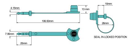
The Acme **G Lock Seal** offers a cost effective solution for the sealing of garment bags in transit or storage. It is manufactured in Acetyl material and can be supplied plain or sequentially numbered. The seal can be supplied with a different coloured cap for easy identification, with or without a company logo. The design incorporates a grooved break-off point for easy removal.
