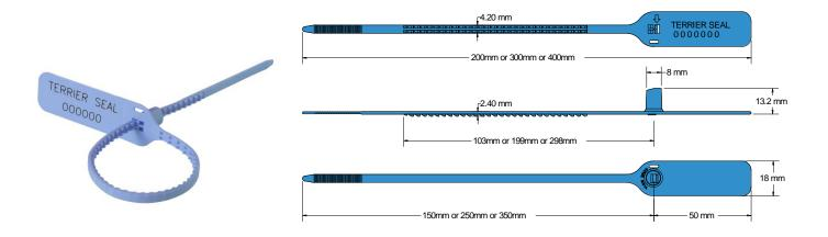
The Acme **Terrier Seal** is a pull tight seal manufactured from Polypropylene material. The strap lock configuration is similar to that of the Combilock seal but is smaller in width and therefore suitable for applications where there is a small sealing aperture and strength is a requirement. This seal is suitable for most applications.
