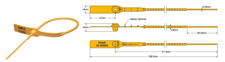
The Acme **Griptight Gen2 Seal** is a heavy duty pull-tight seal manufactured from two dissimilar materials. The acetyl insert is durable and will withstand freezing and boiling conditions, whilst the nylon body is flexible for easy use. The design features rolled heat staking technology to secure the insert to the body, which provides clear evidence of tampering if forced open or cut. This seal is suitable for most applications where strength is a requirement.
