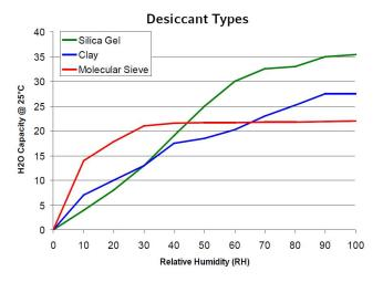
Desi Pak is Clariant's natural bentonite desiccant offering excellent adsorption capacity, even compared to silica gel in low relative humidity packaging environments.
